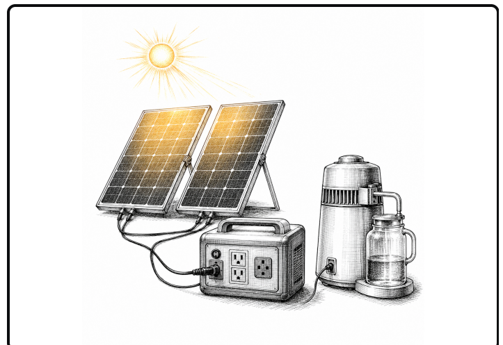
Two 400 watt panels and a power station run the still with no grid.
