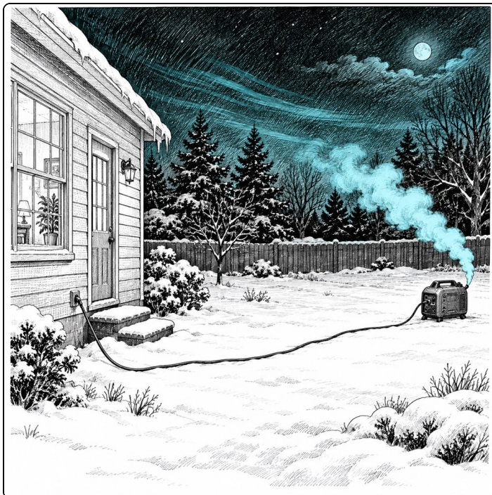
Out in the yard, far from the house, exhaust drifting away from every window and door.
