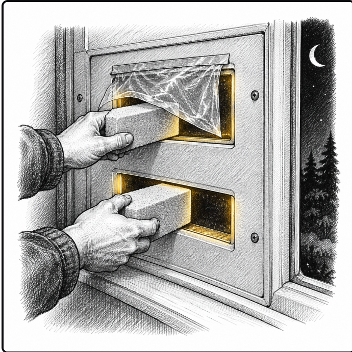
The night damper: a garbage bag flap on the top vent, foam plugs in both.
