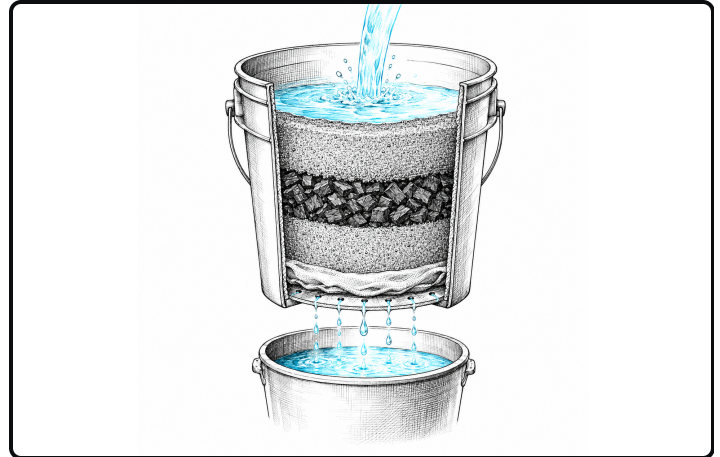
Cutaway: cloth, sand, charcoal, sand. It clears the water, it does not make it safe.
